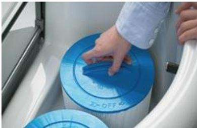
**Step 4:** Using a garden hose with a nozzle or other high-pressure device, clean cartridge(s). Work top to bottom on each pleat.
